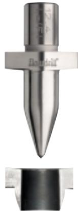
The Flowdrill® Thermal Friction Drill produces perfectly formed bushes using a combination of speed of rotation and pressure to locally heat the material, forming a bush in various thickness of metal.
